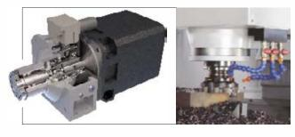
Directly coupled to the ball screws AC servo motors along all axes.
