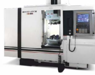
Linear guideways along the three axes - size 25, zero clearance. Stable cutting under full load conditions. Minimum friction when in motion. High precision and high speed with no need for adjustment during operational life.
