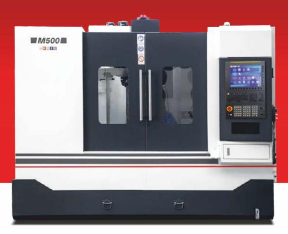
Cartridge type spindle, without need of maintenance. High precision bearings (P4 class). The increased axial tighting force eliminates vibrations at heavy cutting conditions.
